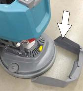
2. Cut cable-tie securing the motor connector harness to machine.
